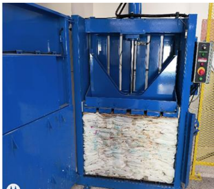
Compactor used to reduce waste volume and optimize residual materials management practices
