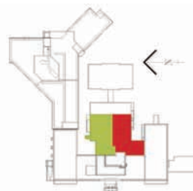
Red: Expansion for MRI Green: Renovations to the existing roof
